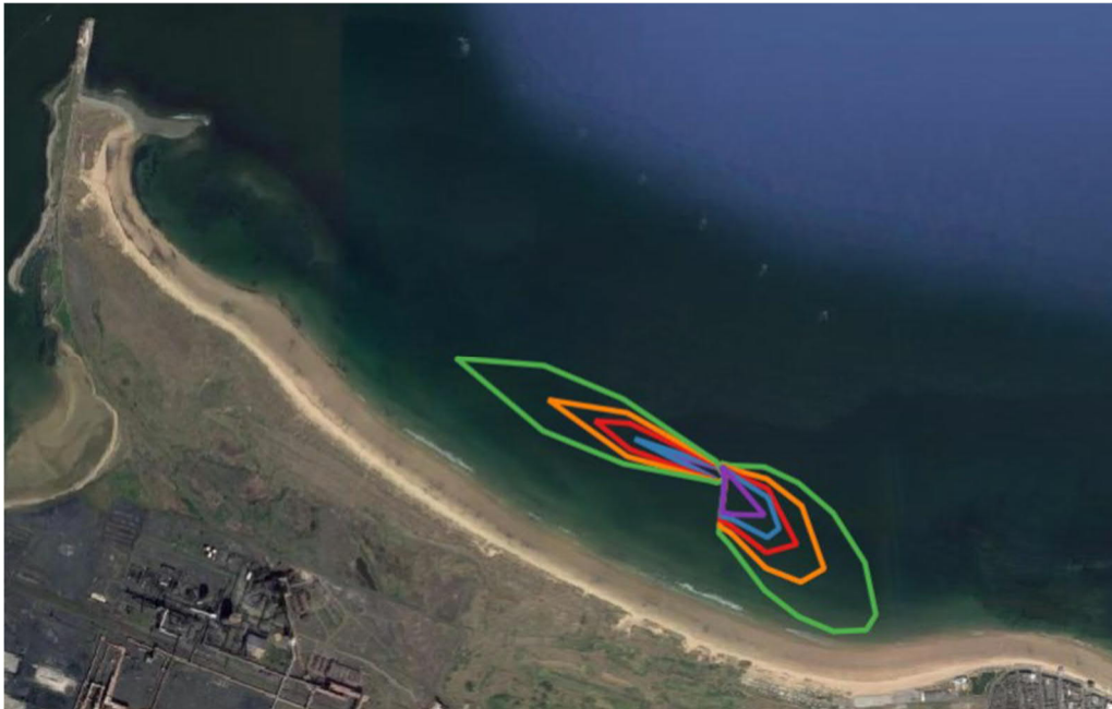
Diagram 14-3: CORMIX Excess Temperature Isolines (°C) During Neap Tide Under Normal Discharge Conditions, at the Replacement Outfall
